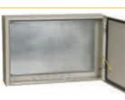
Metal enclosure<br>SCHMP-4.6.1-0 74 U2 IP54 | Casing, mm: 400×600×150<br>Panel, mm: 330×530<br>No. of entries:<br>6 holes diam. 28 mm (bottom).<br>Weight: 12.2 kg    | RAL 7032 | YKM40-461-54 |
