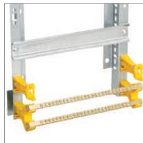
N and PE buses are fixed to the stand holders that are installed into the mounting profile slots with the help of latches.
