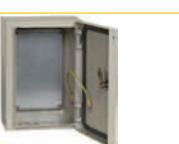
Metal enclosure<br>SCHMP-3.2.1-0 74 U2 IP54  | Casing, mm: 300×210×150<br>Panel, mm: 230×140<br>No. of entries:<br>6 holes diam. 28 mm (bottom).<br>Weight: 3.4 kg     | RAL 7032 | YKM40-321-54 |
