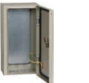
Metal enclosure<br>SCHMP-4.2.1-0 74 U2 IP54 | Casing, mm: 400×210×150<br>Panel, mm: 330×140<br>No. of entries:<br>6 holes diam. 28 mm (bottom).<br>Weight: 4.3 kg     | RAL 7032 | YKM40-421-54 |
