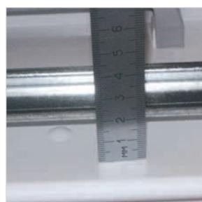
Convenient mounting and cabling: wide space between the DIN-rail and back wall (from 20 to 35 mm). Distance between the different DIN-rails ranges from 125 to 130 mm.
