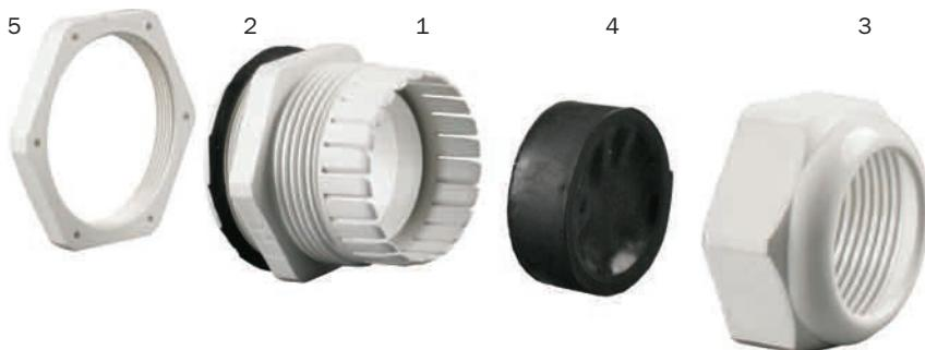
The gland consists of a body (1), sealant (2), a sealing nut (3), a spacer (4) and a clamping nut (5).
