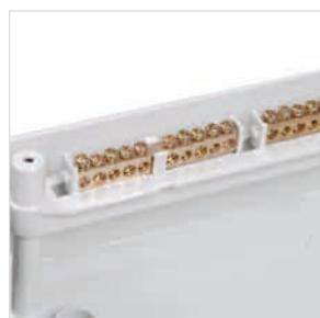
Dismountable N and PE bus holder can be installed both from top and on bottom of the case. N and PE buses are mounted onto a removable holder by a simple latching into mounting faces.
