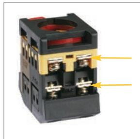
Conductors are connected with screw clamps with disk spring washers ensuring stable fixation.
