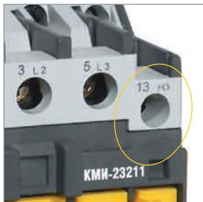
Integrated auxiliary contacts. Each contactor up to 32 A is supplemented with an auxiliary contact: 1 NO or 1 NC. Contactors from 40 up to 95 A are completed with two auxiliary contactors: 1 NO+1 NC.
