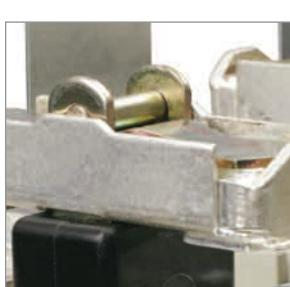
Contact pieces are coated with silver providing for using them in continuous running duty. Welding depositions on the contact pieces are made of silver-based composite materials providing for lowering contact resistance if the temperature rises.
